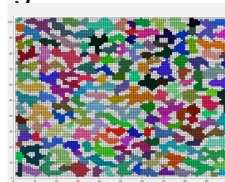
Microstructure Simulation: 40,000 MC steps
